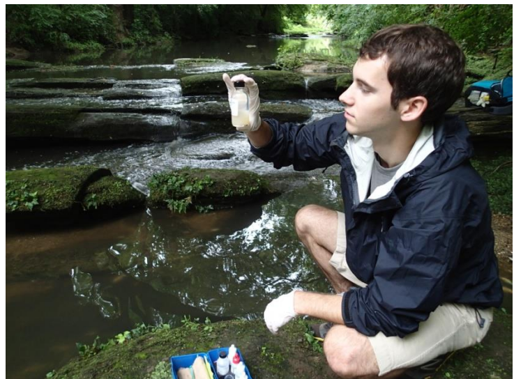
NWW intern Taylor Spear uses a LaMotte test kit to confirm low dissolved oxygen after a major fish kill in Tanyard Creek.
