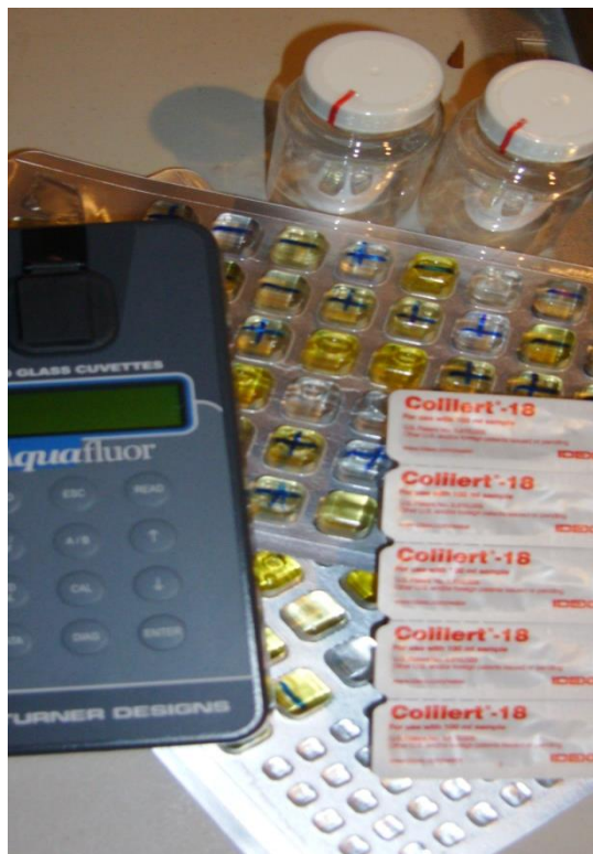
IDEXX® Supplies and a Turner Designs fluorometer, which measures optical brighteners.
