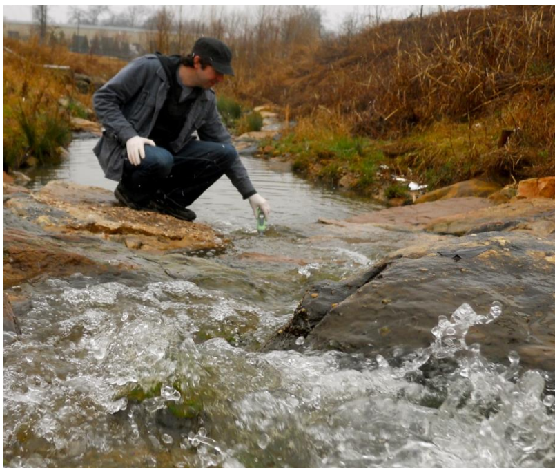
CRK headwaters staff tests Flat Creek with hand-held conductivity probe.
