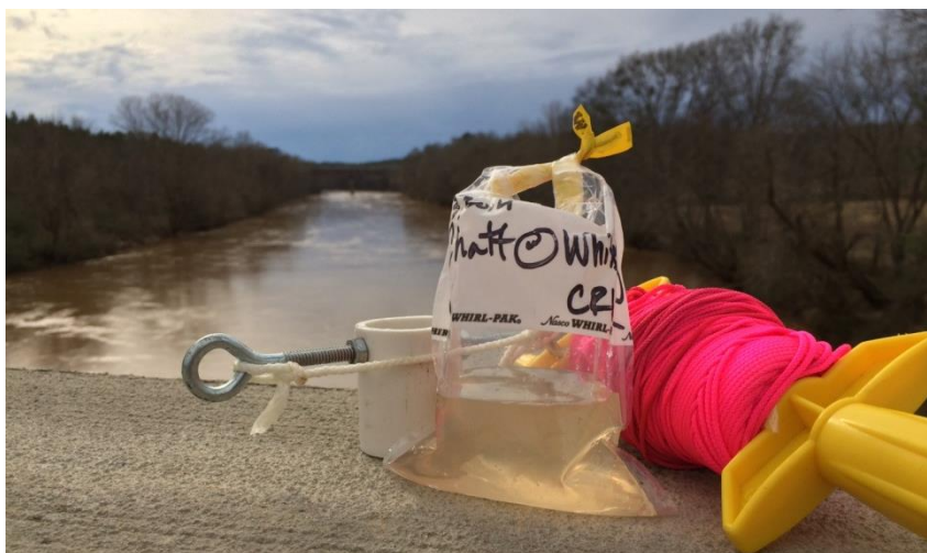
A sample collected from the Chattahoochee River near Whitesburg using a PVC bridge sampler.
