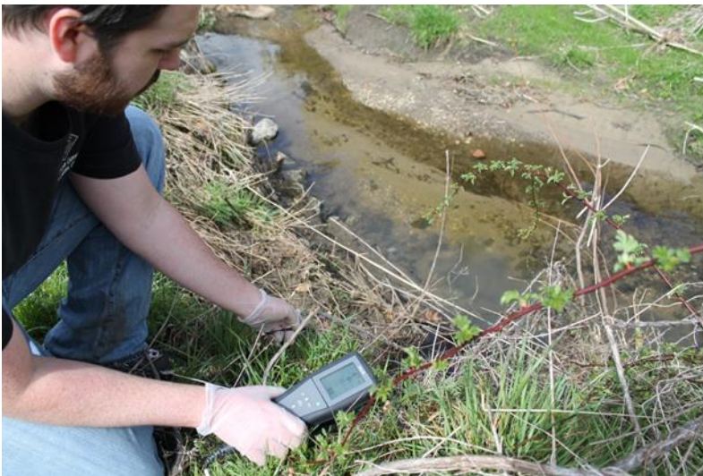
NWW intern uses probe to measure dissolved oxygen at a potential sewer spill in Piedmont Park.
