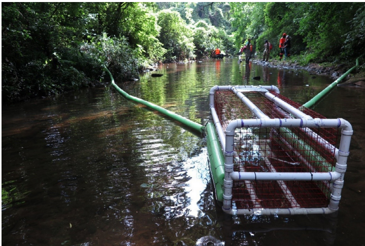
Figure 2: Prototype “Litter Gitter” trash trap along Proctor Creek at Maddox Park, June 2019
