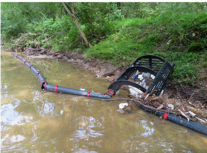
Storm Water Systems "Bandit" trap after anchor failure
